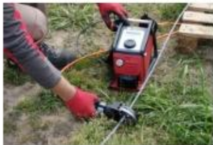
Strand or wire rope cutting in the field
