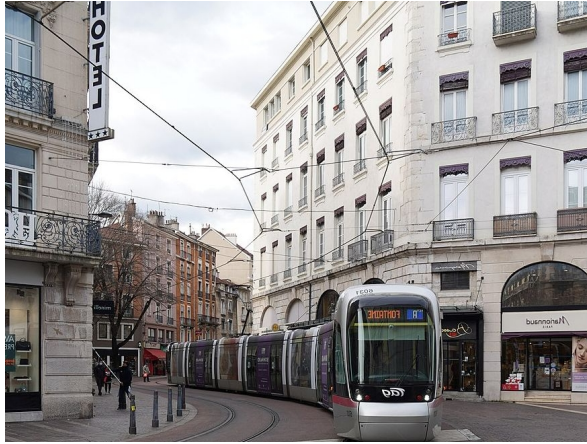
Anchoring of the supporting cable of subway, tramway and trolleybus catenary line (OHL).
