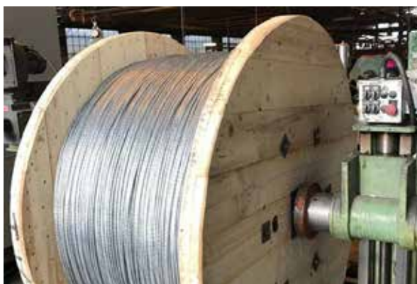
STANDARD Wooden reels from 1000 to 4000 m
