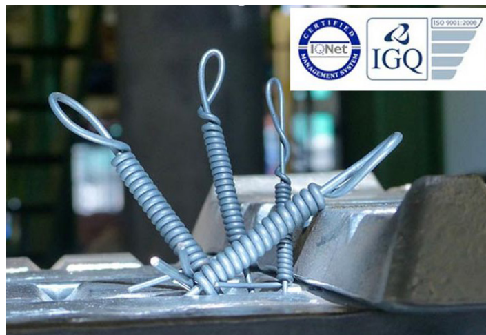
Wrapping test: ductility and adherence
