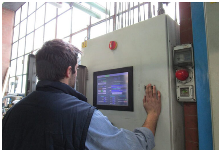
Computerized control of the coating
